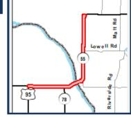
Sealcoat State Highway 55 from the junction with US Highway 95 at Ion Junction in the City of Marsing to Hoskins Road in Canyon County. The treatment will improve ride quality and extend the pavement lifespan. (59% Canyon County and 41% Owyhee County)
