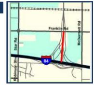
Construct new segment of State Highway 16 from Interstate 84 to Franklin Road in the City of Nampa. Improvements include a new interchange across Interstate 84 with on and off ramps from Interstate 84 to Franklin Road and on to State Highway 16. Design and right-of-way budgeted in separate, previous project (KN 20788).
