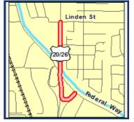
Construct a 10-foot separated, concrete, low-stress multi-use pathway at the interchange of South Broadway Avenue (US 20/26) and South Federal Way in the City of Boise. Project will provide bicycle and pedestrian connectivity and make the area compliant with Americans with Disabilities Act requirements.
