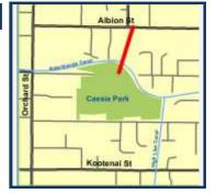
Construct a multi-use pathway adjacent to the existing Electric Light Switch Lateral channel between Cassia Park and Albion Street in the City of Boise. Work includes piping the existing lateral channel and constructing a multi-use bridge over the Ridenbaugh Canal in the southern portion of the pathway corridor to connect this pathway to the ACHD Cassia Street Bikeway and Cassia Park.
