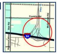
Construct improvements on State Highway 16 from Interstate 84 to Franklin Road, including free flowing ramps at Interstate 84, and a new bridge over Franklin Road in the City of Nampa. These improvements complete the system interchange with Interstate 84 and the Franklin Road interchange.
