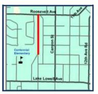
Construct a 12-foot pathway in the center of the alley that extends from South State Street to West Roosevelt Avenue connecting to a 10-foot pathway traversing the eastern boundary of Centennial Elementary School (an extension of South State Street) in the City of Nampa. The project includes drainage on both sides of the pathway, speed humps, signage, and a crosswalk with a Rectangular
