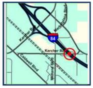
Preliminary engineering and right-of-way acquisition to widen the Karcher Interchange on Interstate 84 in the City of Nampa. Work will include adding a free running right turn lane on the westbound to southbound off-ramp and continue the additional lane across the Interstate 84 and Union Pacific Railroad/Indian Creek structures. The third westbound lane on State Highway 55 to be terminated prior to Middleton Road. Construction will be broken out into separate key numbers.
