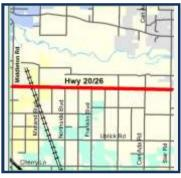
Widen eastbound US 20 from Middleton Road near the City of Caldwell to Star Road near the City of Star. Improvements include two travel lanes in each direction and a center turn lane with two way left turns. Intersection improvements at the mile will include signalization.
