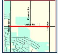
Widen Ustick Road from Franklin Boulevard to 11th Avenue in the City of Nampa from two lanes to four lanes with a raised median. Work includes adding curb, gutter, a multi-use pathway, and Americans with Disabilities Act (ADA) ramps. Facilitated U-Turns are anticipated at the guarter miles to allow vehicles to safely travel in either direction.
