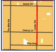
Widen Linder Road from Pine Avenue to Ustick Road in the City of Meridian from two lanes to five lanes (two through-lanes in each directions, center median, and turn pockets where appropriate). Project includes pedestrian and bicycle facilities on both sides of the roadway.
