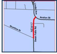
Widen Swan Falls Road from Shortline Street to Avalon Street in the City of Kuna from two lanes to five lanes. Work includes pedestrian and bicycle facilities and replacing and widening a 1940's bridge over Indian Creek from two lanes to four lanes. (Concept level design only. Full design and construction are currently unfunded.)
