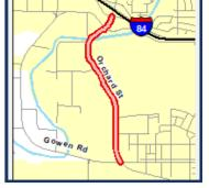
Realign and widen Orchard Street from Gowen Road to Victory Road in the City of Boise to five lanes (two through-lanes in each direction, center median, and turn pockets where appropriate). Project includes enhanced pedestrian and bicycle facilities on both sides of the roadway.
