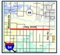
Preliminary engineering and right-of-way acquisition to widen US 20/26 from Middleton Road in the City of Caldwell to Star Road in Ada County. Work will include widening the corridor from two lanes to five lanes (two through lanes each direction and a center turn lane). Intersection improvements will include signalization at the mile. Construction funding is included in KN ORN24309 and ORN24310.
