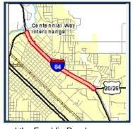
Widen and provide safety improvements on Interstate 84 between the Centennial Way Interchange (Exit 27) and the Franklin Road Interchange (Exit 29) in the City of Caldwell. Work includes an additional lane in each directon and select auxiliary lanes, 10th Avenue Interchange widening and ramp improvements, and drainage improvements.
