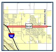
Widen US 20/26 (Chinden Boulevard) from Interstate 84 to Middleton Road to six lanes in the City of Caldwell. Work includes a continuous median traffic separator with u-turn opportunities, and installation of two additional traffic signals.
