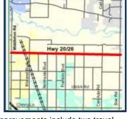
Widen eastbound US 20 from Middleton Road near the City of Caldwell to Star Road near the City of Star. Improvements include two travel lanes in each direction and a center turn lane with two way left turns. Intersection improvements at the mile will include signalization.
