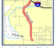
Realign and widen Orchard Street from Gowen Road to Victory Road in the City of Boise to five lanes with enhanced pedestrian and bicycle facilities on both sides of the roadway. Project includes three roundabouts and reconstruction of the Orchard Street and Gowen Road
