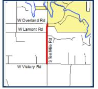
Widen Ten Mile Road, from Victory Road to Overland Road in the City of Meridian, to five lanes with curb, gutter, sidewalk, and level three bicycle facility.
