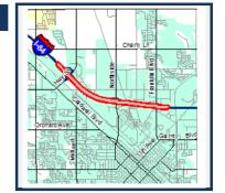
Reconstruct and widen the eastbound and westbound shoulders o Interstate 84 from the Karcher Road Interchange (Midland Boulevard) to the Franklin Boulevard Interchange in the City of Nampa to provide sufficient pavement to temporarily shift traffic during the Interstate 84 reconstruction projects. Design for this project is shown under Key Number 20315.
