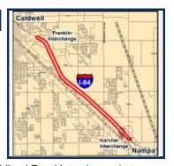
Reconstruct and widen the eastbound lanes of Interstate 84 from the Franklin Interchange to the Karcher/Midland Road Interchange between the City of Caldwell and the City of Nampa in Canyon County. The project includes widening the existing four-lane section (two-lanes each direction) to a six-lane section (three-lanes each direction). This project includes replacement of the Notus Canal bridge structure just west of Ustick Road, Design was programmed under Key Number 22196.
