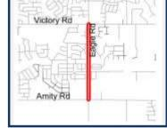
Widen Eagle Road from Amity Road to Victory Road in the City of Meridian to five lanes with curb, gutter, sidewalk, and level three bike lanes. Project includes enhanced pedestrian crossing facility at Rome Drive and a roundabout at Eagle Road and Zaldia Drive.
