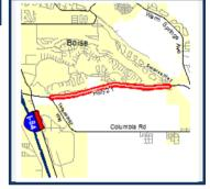
Widen State Highway 21 from Technology Way (near Micron) to Surprise Way (just west of the Boise River Bridge) in the City of Boise. The project includes two 12-foot travel lanes, a continuous 14-foot center turn lane, and two 6-foot shoulders.
