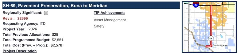
Sealcoat the pavement surface on State Highway 69 (Meridian Road), from Orchard Avenue in the City of Kuna to Interstate 84 in the City of Meridian, to improve ride quality and extend the pavement lifespan.
