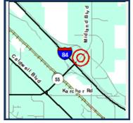
Preliminary engineering and right-of-way acquisition to widen the Karcher Interchange on Interstate 84 in the City of Nampa. Work will include adding a free running right turn lane on the westbound to southbound off-ramp and continue the additional lane across the Interstate 84 and Union Pacific Railroad/Indian Creek structures. The third westbound land on State Highway 55 to be terminated prior to Middleton Road. Construction will be broken out into separate key numbers.
