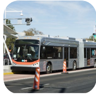
Bus rapid transit (BRT) – exclusive guideway (center)
