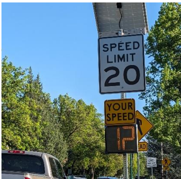
Dynamic Speed Feedback Signs: Alerts drivers of their speed and indicates that their speeds are being monitored and enforcement may be present. Should be implemented in conjunction with other speed management strategies. Most effective when permanently installed and at locations with perceived need to slow. (e.g., school zones)
