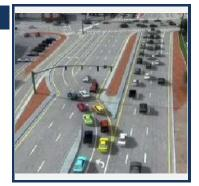
Project Description : Construct a partial continuous flow intersection (CFI), including displaced leftturn lanes, at SH-44 (State Street) and SH-55 (Eagle Road) in the City of Eagle.
