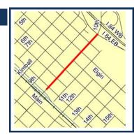
Project Description : Overlay a one-half mile section of 10th Avenue in downtown Caldwell from the railroad overpass to I-84 to replace surface in poor condition. Install intelligent transportation system (ITS) components and bring pedestrian facilities to current standards.
