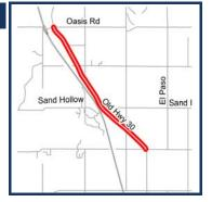
**Project Description :** Rehabilitate Old Highway 30 from the vicinity of Goodson Road to Oasis Road, located north of the City of Caldwell in Canyon County, with a cement recycled asphalt base to improve the road condition.
