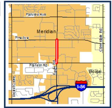
**Project Description :** Construct a lighted ten-foot-wide concrete multi-use pathway along the east side of State Highway 55 (Eagle Road) from Franklin Road to Pine Avenue in the City of Meridian. Reconstruct the existing sidewalk adjacent to the Shell gas station to the ten-foot width. The project will include an eight-foot separation between the roadway and pathway where possible.
