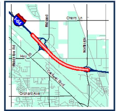
**Project Description :** Reconstruct and widen I84 from Northside Boulevard Interchange to the Karcher Road Interchange (Midland Boulevard) in the City of Nampa. The project includes widening the existing four-lane section (two lanes each direction) to an eight-lane section (three lanes each direction plus auxiliary lanes between Northside Boulevard and the Karcher Road Interchanges). Design for this project is shown under Key Number 20315.
