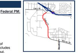
Project Description: Realign and widen Orchard Street from Gowen Road to I-84 in the City of Boise to five lanes with curb, gutter, sidewalk, and bike lanes. Project includes reconstruction of the Gowen Road intersection as a multi-lane roundabout.
