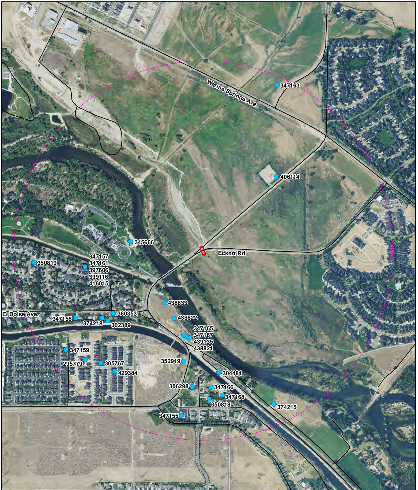
Figure 6. Well Records Within 1/2 Mile of the Eckert Road Underpass Project.
