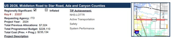
Preliminary engineering and right-of-way acquisition to widen US 20/26 from Middleton Road in the City of Caldwell to Star Road in Ada County. Work will include widening the corridor from two lanes to five lanes (two through lanes each direction and a center turn lane). Intersection improvements will include signalization at the mile. Construction will be broken out as funding is determined.
