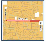
Widen Ustick Road from Ten Mile Road to Linder Road in the City of Meridian to five lanes. The projects includes curb, gutter, sidewalk, and a level three bicycle facility. The concept-level design will further clarify the scope of the project.
