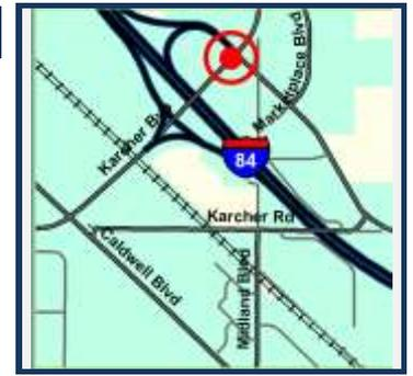
Preliminary engineering and right-of-way acquisition to widen the Karcher Interchange on Interstate 84 in the City of Nampa. Work will include adding a free running right turn lane on the westbound to southbound off-ramp and continue the additional lane across the Interstate 84 and Union Pacific Railroad/Indian Creek structures. The third westbound lane on State Highway 55 to be terminated prior to Middleton Road. Construction will be broken out into separate key numbers.
