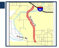
Realign and widen Orchard Street from Gowen Road to Victory Road in the City of Boise to five lanes with enhanced pedestrian and bicycle facilities on both sides of the roadway. Project includes three roundabouts and reconstruction of the Orchard Street and Gowen Road intersection.
