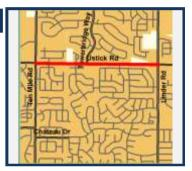
Widen Ustick Road from Ten Mile Road to Linder Road in the City of Meridian to five lanes. The project includes curb, gutter, sidewalk, and a level three bicycle facility. The concept-level design will further clarify the scope of the project.
