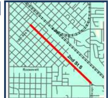
Install 19 high efficiency roadway street lights along 2nd Street South from 16th Avenue South to Chicago Street; two Rectangular Rapid Flashing Beacon (RRFB) crossings, a Left Turn Lane and a Two-Way-Left-Turn-Lane (TWTL) with roadway reconstruction from 16th Avenue South to 24th Avenue South; and provide a five-foot paved shoulder (at least four-feet) along the south side of 2nd Street South from 24th Avenue South to Chicago Street, in the City of Nampa.
