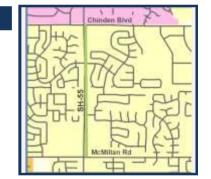
Design and construct a 10- to 12- foot detached multi-use pathway adjacent to State Highway 55 (Eagle Road) on the east side between McMillan Road and US 20/26 (Chinden Boulevard) in the City of Boise. Improvements include widening existing pathway and filling gaps where a pathway is missing. The pathway will increase the safety of bicyclists and pedestrians along the corridor.
