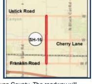
Construct new segment of State Highway 16 from Franklin Road to Ustick Road the City of Nampa and Canyon County. The roadway will include two lanes in each direction with at-grade intersections at Franklin Road and Ustick Road utilizing the on and off ramps for the future interchanges. Work also includes a new structure over the Union Pacific Railroad, Cherry Lane, Ten Mile Creek, and irrigation structures. Design and right-of-way budgeted in separate, previous project (KN 20788).
