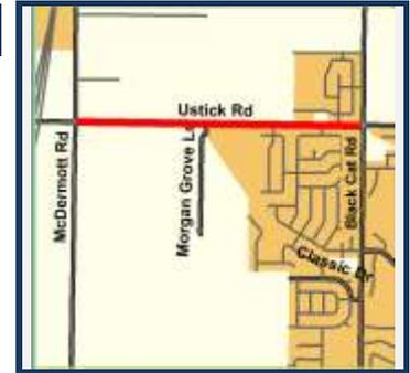
Widen Ustick Road from two lanes to five lanes from McDermott Road to Black Cat Road in the City of Meridian including enhanced pedestrian and bicycle facilities on both sides of the roadway.
