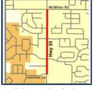
Design and construct a ten-foot wide multi-use pathway adjacent to State Highway 55 (Eagle Road) on the west side between Jasmine Lane to McMillian Road. Improvements include widening existing pathway and filling gaps where a pathway is missing. The pathway will increase the safety of bicyclists and pedestrians along the corridor.
