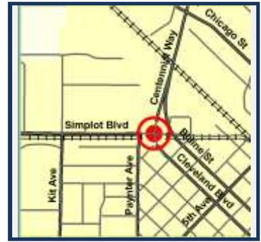
Replace a six-legged intersection at State Highway 19 (Simplot Boulevard) and Interstate 84-B (Centennial Way, Cleveland Boulevard, and Blaine Street) with a roundabout intersection in the City of Caldwell.
