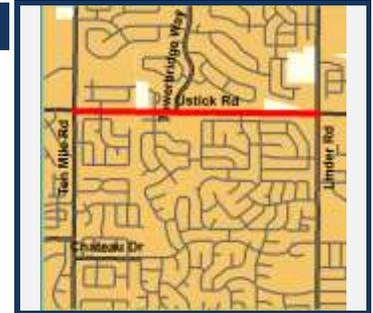
Widen Ustick Road from Ten Mile Road to Linder Road in the City of Meridian to five lanes. The project includes curb, gutter, sidewalk, and a level three bicycle facility. The concept-level design will further clarify the scope of the project.
