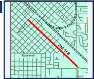
Install 19 high efficiency roadway street lights along 2nd Street South from 16th Avenue South to Chicago Street; two Rectangular Rapid Flashing Beacon (RRFB) crossings, a Left Turn Lane and a Two-Way-Left-Turn-Lane (TWTL) with roadway reconstruction from 16th Avenue South to 24th Avenue South; and provide a five-foot paved shoulder (at least four-feet) along the south side of 2nd Street South from 24th Avenue South to Chicago Street, in the City of Nampa.
