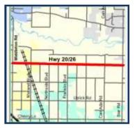
Widen westbound US 20 from Middleton Road near the City of Caldwell to Star Road near the City of Star. Improvements include two travel lanes in each direction and a center turn lane with two way left turns. Intersection improvements at the mile will include signalization.
