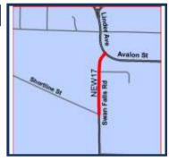
Widen Swan Falls Road from Shortline Street to Avalon Street in the City of Kuna from two lanes to five lanes. Work includes pedestrian and bicycle facilities and replacing and widening a 1940's bridge over Indian Creek from two lanes to four lanes. The project is in early development and the cost and timing are not yet known.
