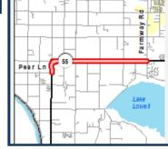
Preliminary engineering and right-of-way acquisition to make capacity and safety improvements to State Highway 55 (Karcher Road) from Pear Lane to Farmway Road in Canyon County. Work includes widening to include two travel lanes in each direction, a continuous center turn lane and wide shoulders for pedestrian and bicycle use. Improvements include bridge replacements, culvert extensions and significant utility relocations.
