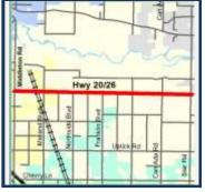
Widen eastbound US 20 from Middleton Road near the City of Caldwell to Star Road near the City of Star. Improvements include two travel lanes in each direction and a center turn lane with two way left turns. Intersection improvements at the mile will include signalization.
