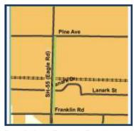
Construct a lighted ten-foot-wide concrete multi-use pathway along the east side of State Highway 55 (Eagle Road), from Franklin Road to Pine Avenue in the City of Meridian. Reconstruct the existing sidewalk adjacent to the Shell gas station to the ten-foot width. The project will include an eight-foot separation between the roadway and pathway where possible.
