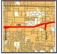
Add an auxiliary lane on Interstate 84 between Meridian Road (Exit 44) and Eagle Road (Exit 46) Interchanges in the City of Meridian, including an additional lane and shoulder on the eastbound on-ramp at Meridian Road and the eastbound off-ramp at Eagle Road. Work includes all studies and design work necessary. Traffic patterns on Interstate 84 from Meridian to the WYE interchange in the City of Boise will also be studied.
