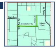
To plan and design pathway connections in the south/central part of the City of Nampa near the intersection of 12th Avenue Road and Greenhurst Road. Work includes designing bicycle and pedestrian facilities along Constitution Way and South Juniper Street. This project is funded through the Active Transportation Infrastructure Improvement Program (ATIIP), a competitive Federal Highway Administration grant. Construction is unfunded.
