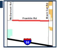
Widen and realign Franklin Road from McDermott Road to Black Cat Road in Ada County from two lanes to five lanes(two through-lanes in each direction, center median, and turn pockets where appropriate). Project includes enhanced pedestrian and bicycle facilities on both sides of the roadway.
