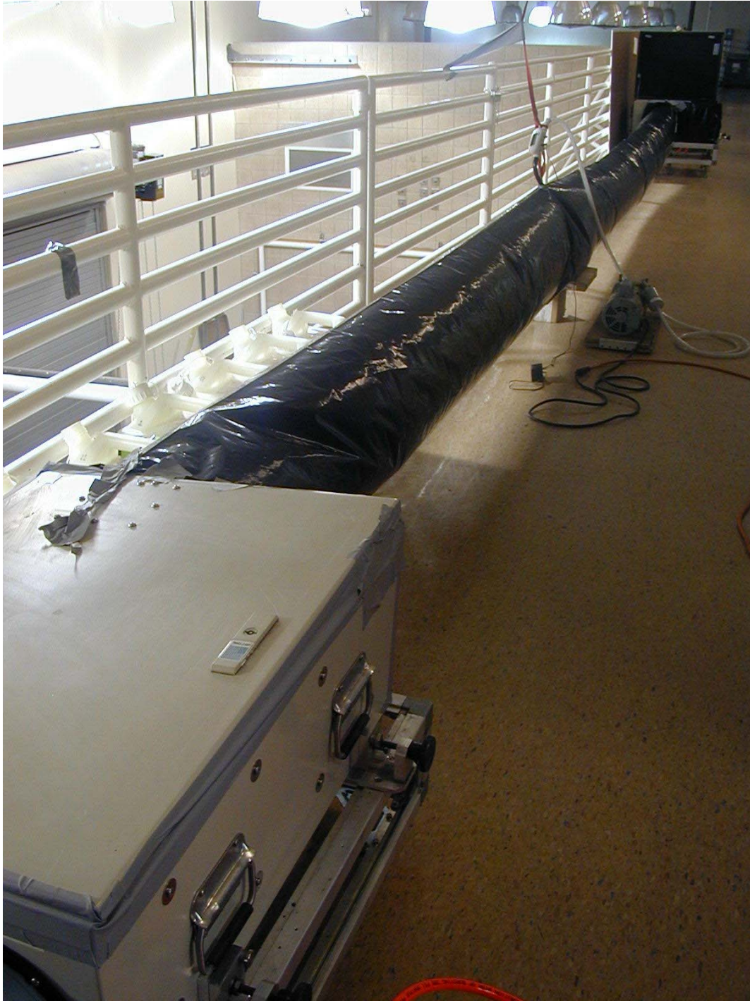
Figure 3-6. LIDAR calibration configuration showing HEPA filtered air inflating the calibration cell (lawn and leaf bag material).
