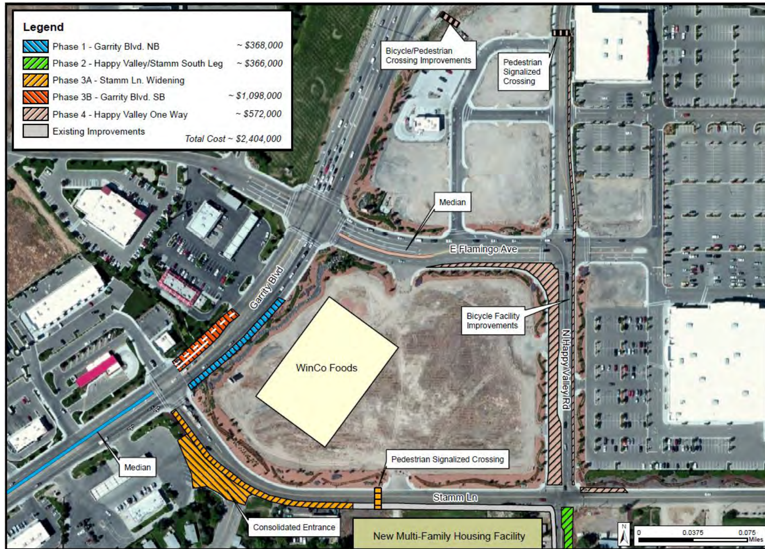
Figure 5. Phasing of Alternative 4 improvements
