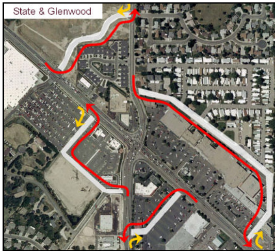
Figure 4-2 Four-quadrant system at State and Glenwood
