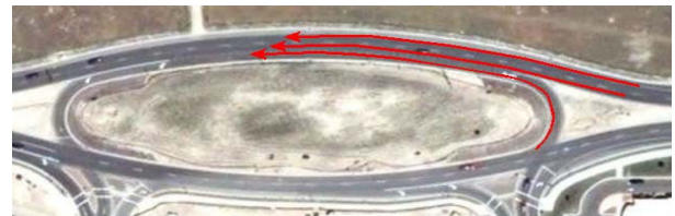
Figure 4-1 Bowtie that avoids impeding oncoming traffic
