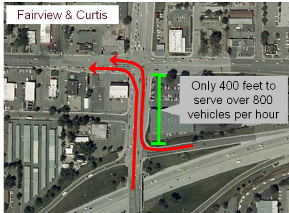
Figure 8-1 Fairview and Curtis: huge demand, no storage space
