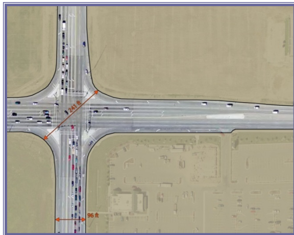
a: Typical Conventional Intersection Footprint
