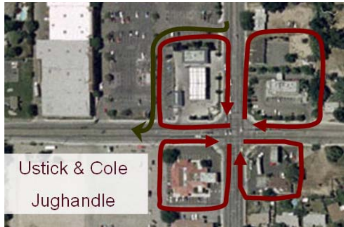
Figure 2-19: Jughandle turn movements
