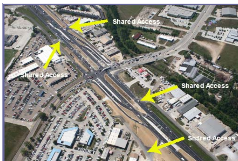
Figure 3-9: Shared Access Near a CFI
