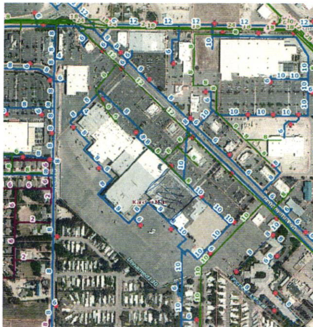
City of Nampa – Karcher Mall Utilities – Blue = Water Green = Sewer Purple = Pressure Irrigation
