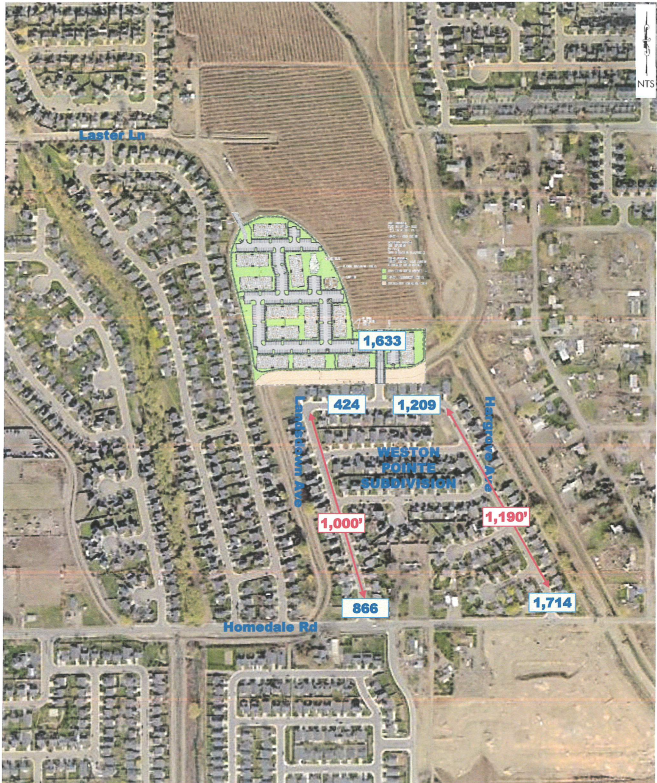
Figure 4.4 – Site Access, Circulation, and ADT
