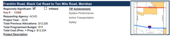
Widen Franklin Road from two-lane to five-lane from Black Cat Road to Ten Mile Road. Work includes curb, gutter, drainage swales, sidewalks, and bicycle facilities, and reconstructing the intersection at Franklin Road and Black Cat Road with a seven-lane by seven-lane intersection.
