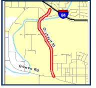
Realign and widen Orchard Street from Gowen Road to Victory Road in the City of Boise to five lanes with enhanced pedestrian and bicycle facilities on both sides of the roadway. Project incudes three roundabouts and reconstruction of the Orchard Street and Gowen Road
