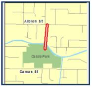
Construct a multi-use pathway adjacent to the existing Electric Light Switch Lateral channel between Cassia Park and Albion Street in the City of Boise. Work includes piping the existing lateral channel and constructing a multi-use bridge over the Ridenbaugh Canal in the southern portion of the pathway corridor to connect this pathway to the ACHD Cassia Street Bikeway and Cassia Park.
