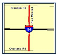
Widen Five Mile Road from Overland Road to Franklin Road in the City of Boise to five lanes including enhanced pedestrian and bicycle facilities on both sides of the roadway. Project costs do not include work on the overpass (see associated project key numbers ORN23591). Design, environmental work, and right-of-way are included in key number 23095.
