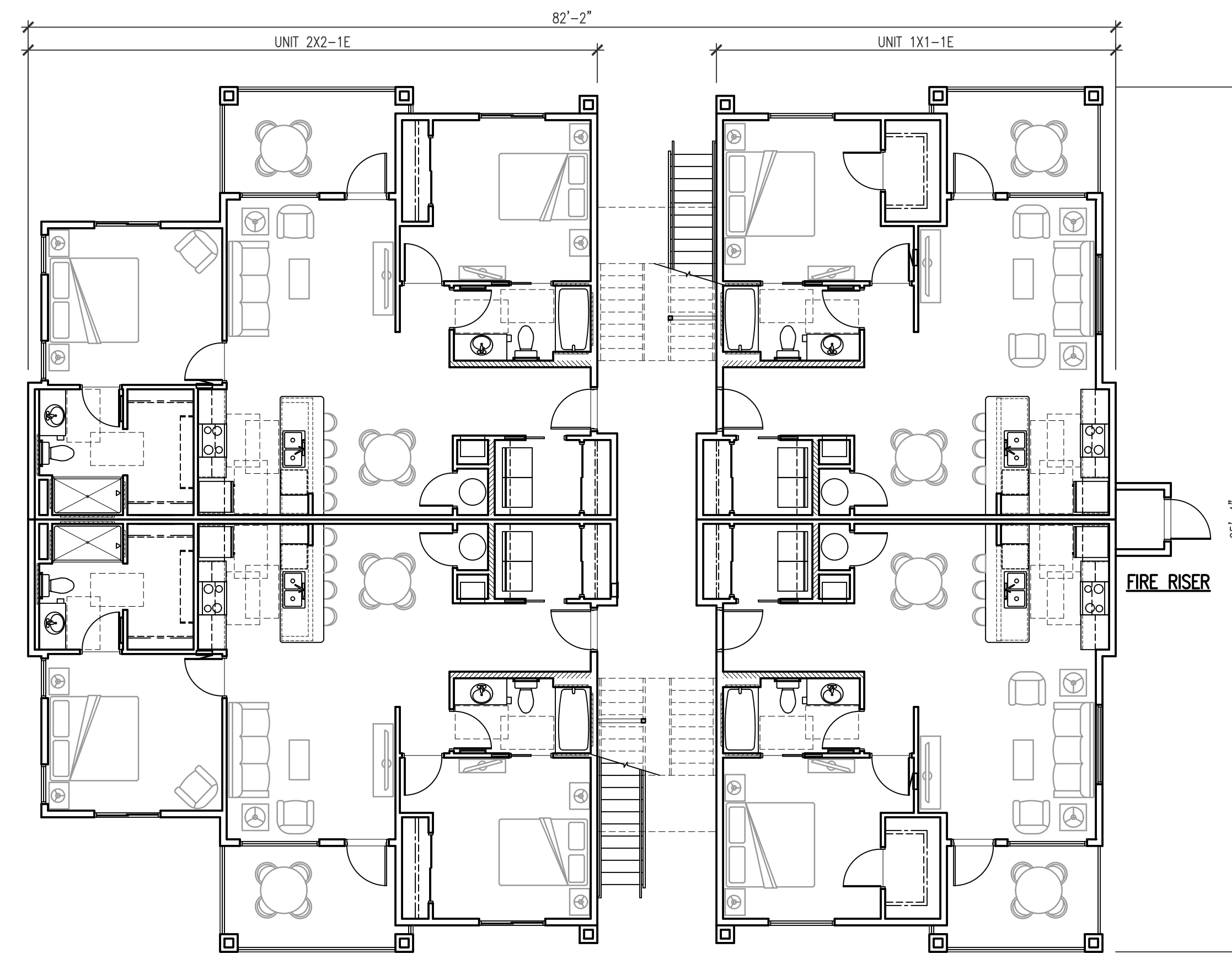
1 BUILDING TYPE 3 (BLDG. A) TYPICAL FLOOR PLAN SCALE: 1/8" = 1'-0" AREA: 4,903 SF PER FLOOR x 3 = 14,709 SF REAR LEFT RIGHT FRONT
