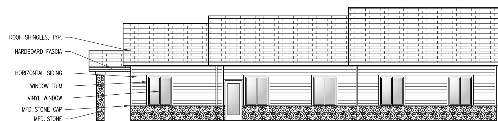
7 NORTH ELEVATION - AMENITY BUILDING SCALE: 1/8" = 1'-0"
