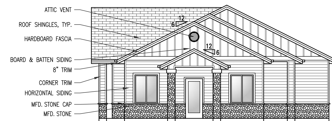
4 EAST ELEVATION - AMENITY BUILDING SCALE: 1/8" = 1'-0"
