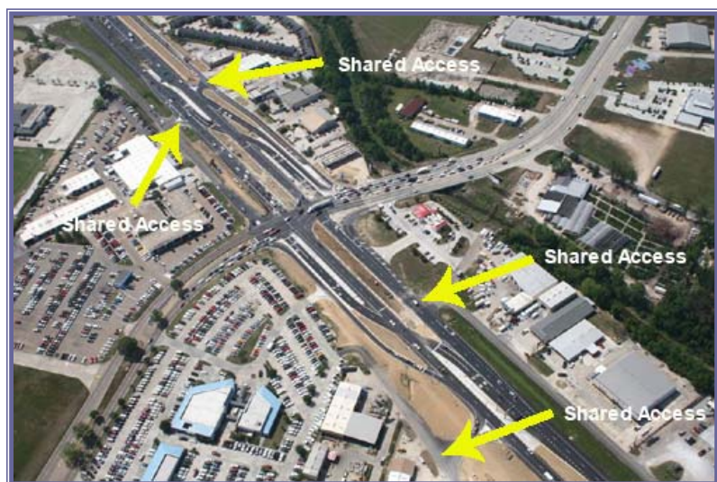
Figure 3-9: Shared Access Near a CFI
