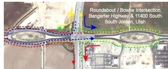
Figure 2-1 Example Bowtie with wrap-around lanes
