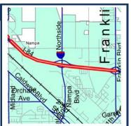
Project Description: Rehabilitate I-84 from the Karcher Interchange (milepost 32) to the Franklin exit in the City of Nampa (milepost 36) to address cracking and poor road conditions. Mill off the existing pavement and add new asphalt, and make improvements to joints.
