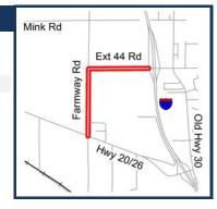
Total Cost (Previous + Programmed): \$2,449 Project Description: Reconstruct Farmway Road, US 20/26 to Extension 44 Road and Extension 44 Road from Farmway Road to I-84 ramps. Work includes eliminating abrupt shoulders and corrects substandard bridge crossings.
