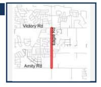
Widen Eagle Road from Amity Road to Victory Road in the City of Meridian to five lanes with curb, gutter, sidewalk, and level three bike lanes. Project includes enhanced pedestrian crossing facility at Rome Drive and a roundabout at Eagle Road and Zaldia Drive.
