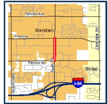
**Project Description :** Construct a lighted 10-foot-wide concrete multi-use pathway along the east side of SH-55 (Eagle Road) from Franklin Road to Pine Avenue in the City of Meridian. Reconstruct the existing sidewalk adjacent to the Shell gas station to the 10-foot width. The project will include an eight-foot separation between the roadway and pathway where possible.
