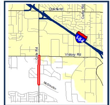
**Project Description :** Widen Cole Road from McGlochlin Street to Victory Road in the City of Boise. Project also includes intersection improvements at Cole Road and Victory Road to six lanes on Victory Road and seven lanes on Cole Road. Project includes widening of a bridge.
