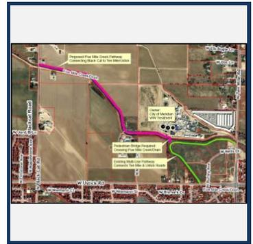
**Project Description :** Design and construct a one-mile segment of the City of Meridian's multi-use pathway extending the current pathway just south of the wastewater treatment plant to Black Cat Road. The project also includes a pedestrian bridge over Five Mile Creek.
