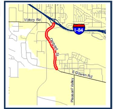
**Project Description :** Realign and widen Orchard Street from Gowen Road to I-84 in the City of Boise to five lanes with curb, gutter, sidewalk, and bike lanes. Project includes reconstruction of the Gowen Road intersection as a multi-lane roundabout. Final alignment will be determined by the Orchard Alignment Study.
