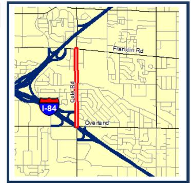
**Project Description :** Widen Cole Road from I-84 to Franklin Road in the City of Boise (formerly KN RD207-16). Project also includes intersection improvements at Cole Road and Franklin Road to seven lanes in all directions. Project will also realign the Cole Road and McMullen Road intersection, reconstruction/widening of a bridge, and improving the existing railroad crossing.
