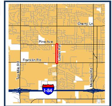
Project Description : Widen Linder Road between Franklin Road and Pine Avenue in the City of Meridian to five lanes, including curb, gutter, sidewalk, and bike lanes. Project includes upgrade of the railroad crossing and replacement and widening of a bridge structure.
