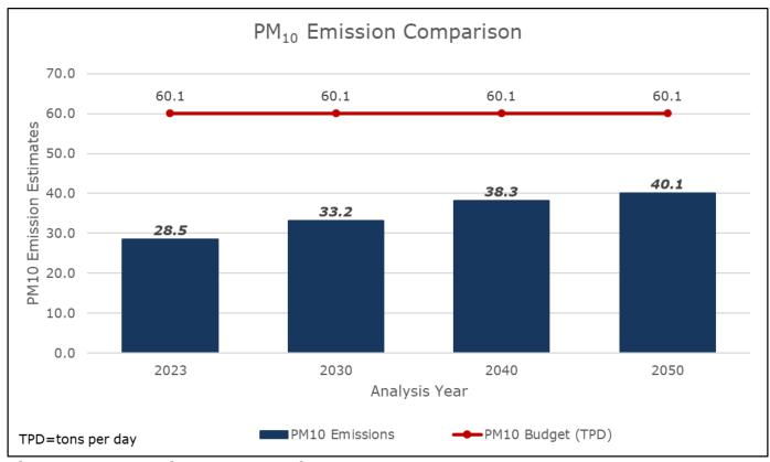
Figure 4: PM<sub>10</sub> Budget Test Results
