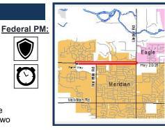
**Project Description :** Widen US 20/26 (Chinden Boulevard) from SH-16 to the existing five-lane section, approximately 700 feet to the west of Linder Road to five lanes (two through lanes in each direction and a two way left center turn lane). The project will include turn lanes and raised medians where necessary. Project funded and constructed by the developer of the Costco shopping center using State Tax Anticipated Revenue (STAR) financing.
